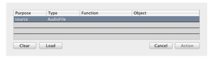
The function started in this example expects a single object of type AudioFile. It's purpose for the function is described as "source". To hand over an appropriate object to the FunctionLoader, select the object in the pool and click on "Load" in the FunctionLoader window. The object will now be handed over to the FunctionLoader and it will show up in the object list:
