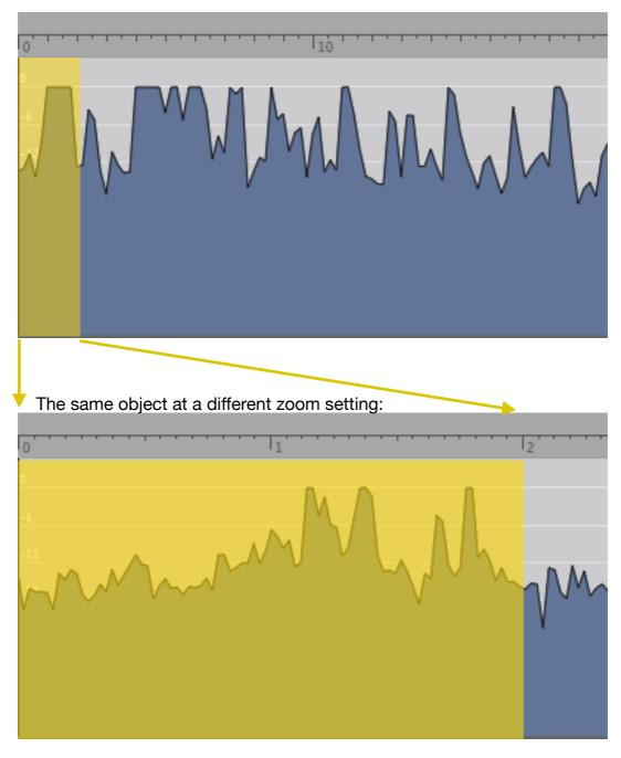
There is a function plug-in called ResampleEnvelope. Use it to limit the resolution of an envelope.
