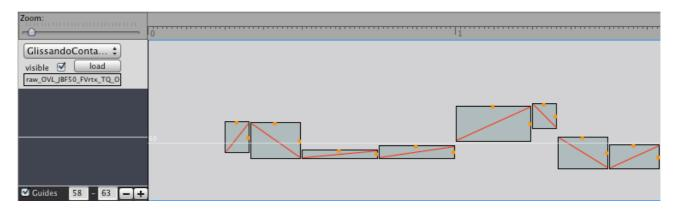
It uses the parameter *pitchF* (a floating point representation of midi pitch) for the positioning of objects on its y-axis, and the parameter *pitchRange* for their height.
