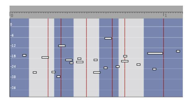
After quantization with the displayed grid, the events are pulled to the grid points. In addition their durations will have changed accordingly:
