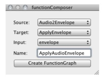
In the FunctionComposer, choose the source and target functions. If the two functions are compatible, possible connecting objects (matching input objects of the target function) will be displayed in the third pop-up (labeled "Input"). In the example above, the function "Audio2Envelope" is being combined with the function "ApplyEnvelope".
