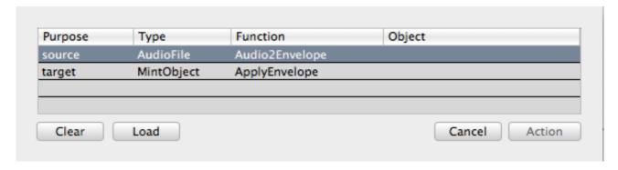
The function *Audio2Envelope* needs an object of type AudioFile, the function *ApplyEnvelope*, in addition to the envelope provided by *Audio2Envelope*, needs an object of type QuinceObject with the purpose "target" on which the envelope should be applied.
